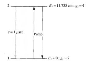
**8.2.** An experiment involving a homogeneously broadened optical amplifier is depicted in the diagram below. For an input intensity of  $1W/cm^2$ , the gain (output/input) is 10 dB. If the input intensity is doubled to  $2W/cm^2$ , the gain is reduced to 9 dB.
